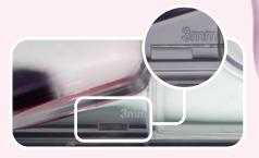
**3mm indicator** on the warming plate as a reference for accurate aspiration of the solutions
